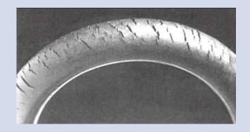
Polymer scission causing brittleness, cracking and loss of strength
