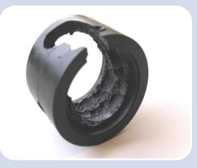
Polymer degradation and loss of functional ingredients causing brittleness, loss of strength and elongation at break
