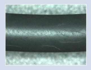
Sudden pressure drop can cause deep cracks in the gasket, as gas is trying to escape:
