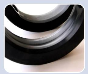
Poor resistance to compression set leads to permanent deformation.
