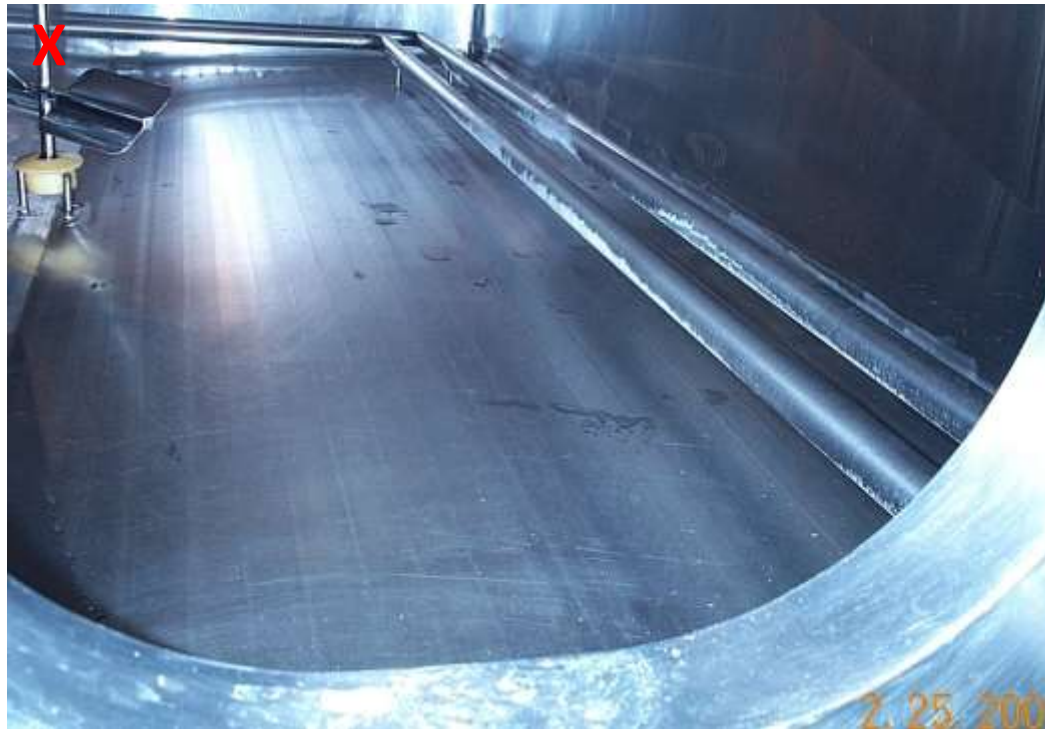
no CIP coverage on bottom of tubes
