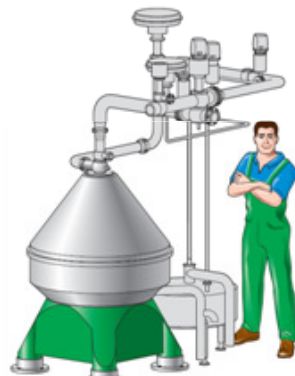
Figure 1 — Typical 2 phase centrifuge with basic piping
