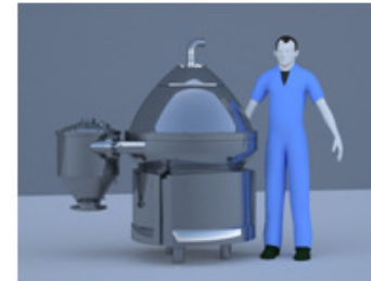
Figure 2 — Typical centrifuge for clarifying
