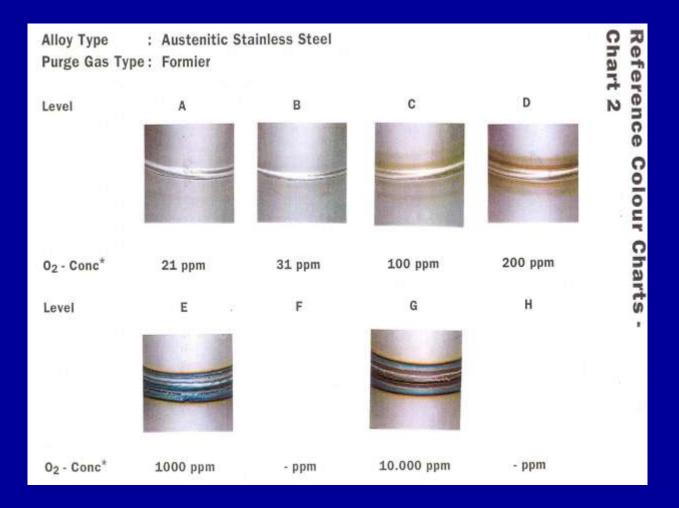
Heat tints on pickled austenitic stainless steel tube butt welds made with *Formier* purging gas (*NH10*) containing known oxygen levels. \* Heat input: 0.2-0.3 kJ/mm.
