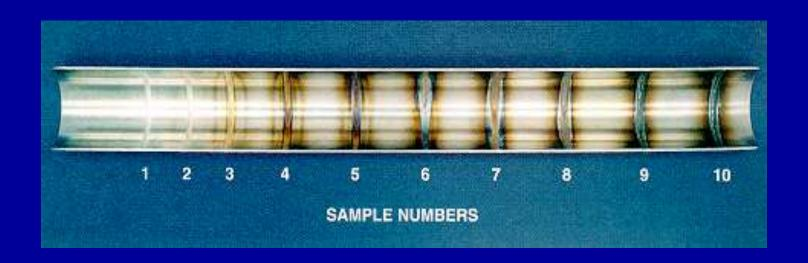
The Sample Numbers refer to the amount of oxygen in the purging gas:
