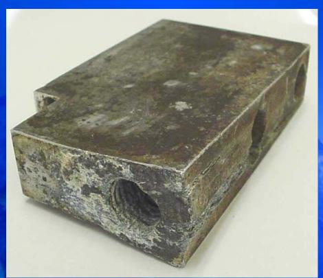
**Bearing Corrosion Salt Brine**
