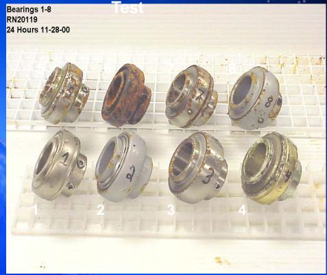
Use aluminum ONLY when necessary, and when so, anodize (or applicable process) to inhibit corrosion and wear.
