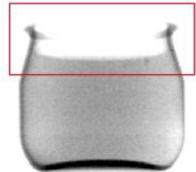
Fill level control in a yogurt cup
