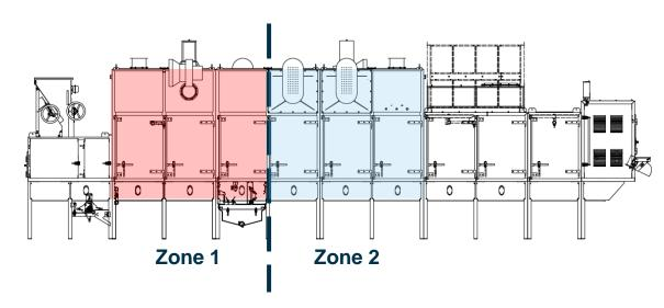
Zone – Referencing a specific dryer area with individually controlled airflow, volume, temperature, exhaust volume, and humidity
